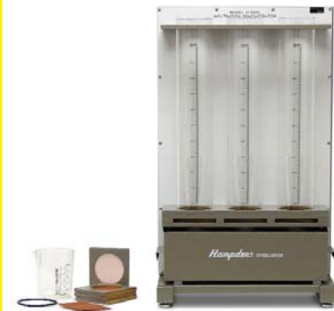
The Model H-6520 Infiltration Demonstrator investigates the infiltration rates of different soil types and soil surface treatments. (Shown with accessories)
