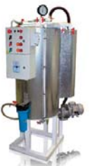
The Model H-BIO-100 Bio Diesel Demonstrator is ideal for the small producer using the same protocol and with the same quality construction as the larger units. Bio Diesel units are chosen for their rugged design, ease of use, no wash process protocol and price/capacity ratio. The H-BIO-100 is capable of producing up to 26.5 gallons per batch.
