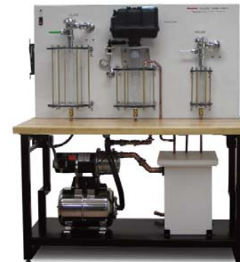
The Model H-RPT-1 Residential Piping Trainer demonstrates the process of a low flow pressure assisted toilet system.
