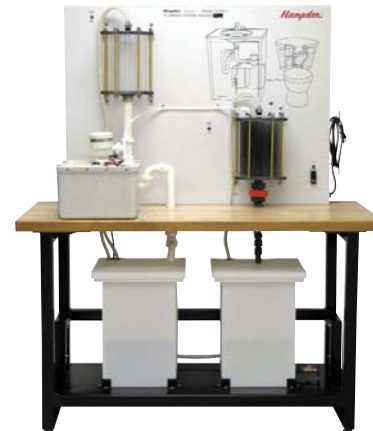
The Model H-PST-1 Plumbing System Trainer demonstrates the process of using gray water in toilet flushing systems.
